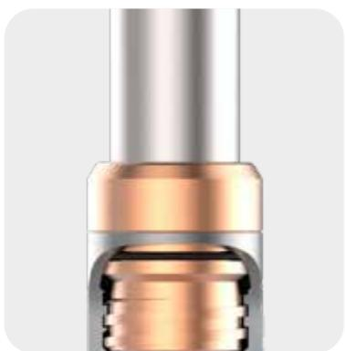
**No gas leaks.** O-ring retention, high temperature seal that prevents the nozzle from loosening and eliminates any loss of gas that occurs in the threads.
