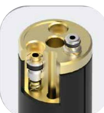
**Liquid loss blockage.** Valves of automatic closing of the cooling circuit, allows to make a quick change of neck without loss of liquid and without the need to stop the cooling group.
