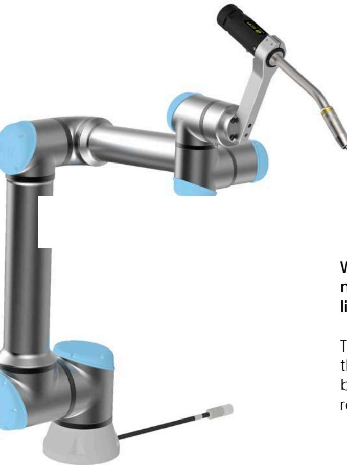
Welding torches designed for collaborative robots do not need anti-collision systems, which makes them lighter and easier to set up.
