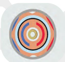
4º-Double circuit cooling system for nozzle and contact tip completely Independent. Gas driving totally separates from the rest of circuits like the thread of contribution, improving the stability of the gas outlet and the projection.
