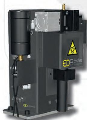
Automatic cleaning station for robotic welding systems.
