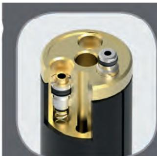
1°-Valves of automatic closing of the cooling circuit, allows to make a quick change of neck without loss of liquid and without the need to stop the cooling group.
